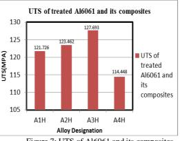
Figure 7: UTS of Al6061 and its composites
