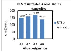
Figure 6: UTS of Al6061 and its composites
