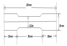
Figure 3: Showing specimen dimensions foe testing UTS (Ultimate Tensile Strength) on UTM.
